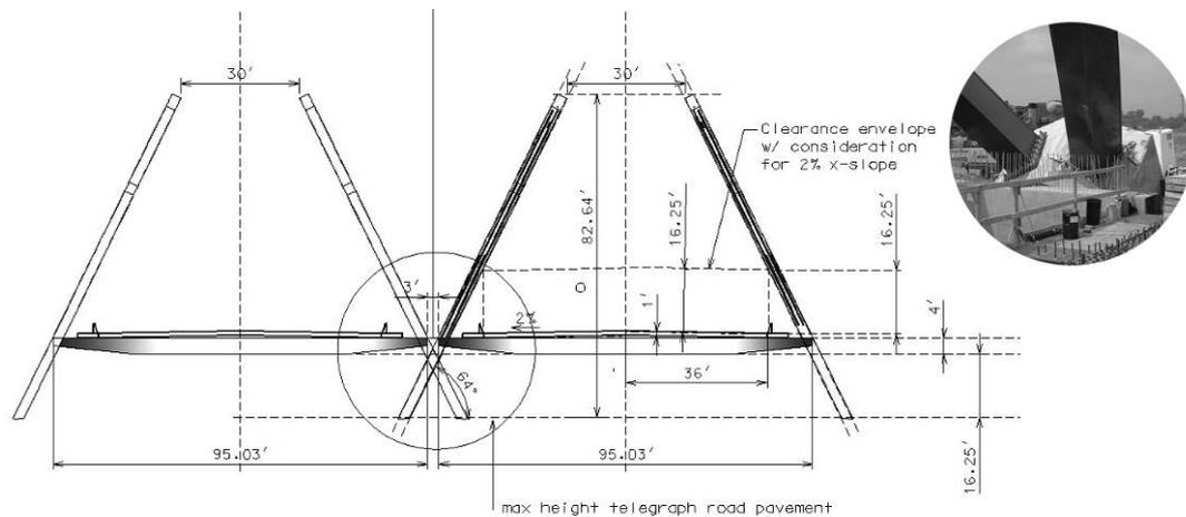
Figure 8 : Unequal Length of arches
