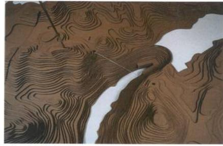
Figure 6 : Wind Tunnel Terrain Model
