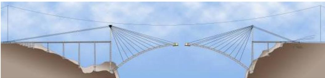
Figure 10 : Stayed Erection Scheme
