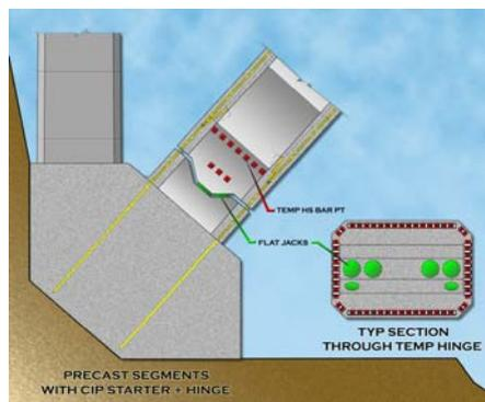
Figure 11 : Precast Segmental Springing Option
