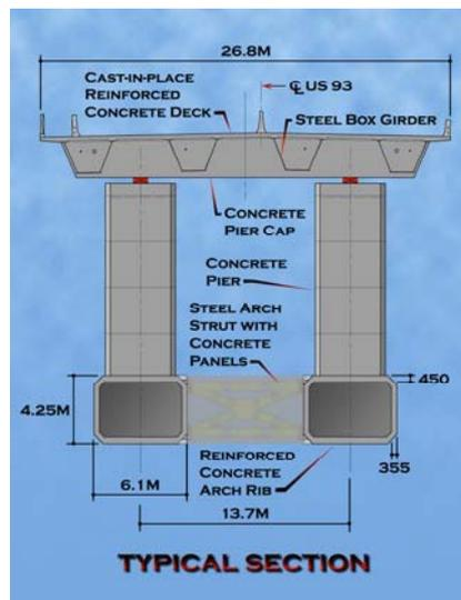
Figure 7 : Arch Framing System
