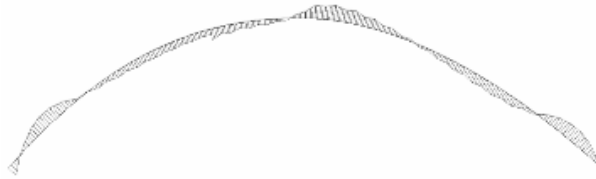
Figure 7 : Moment distribution diagram of arch rib in built bridge period (left y = x^{2.4} , right y = x^{1.8} parabola)
