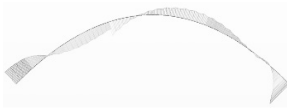
Figure 6 : Distribution diagram of arch rib moment in built bridge period (Quadratic Parabola)
