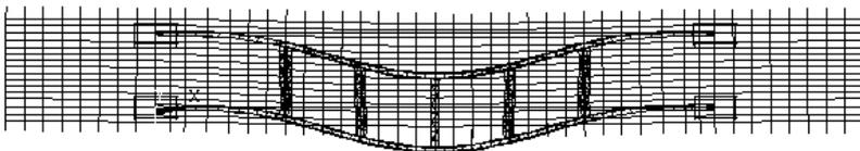
Figure 7: Collapse modal under maximum moment at crown
