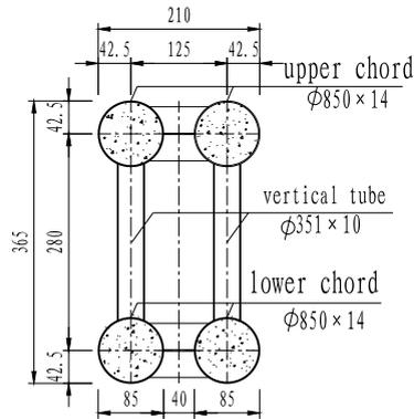
Fig. 4: Cross section of arch rib
