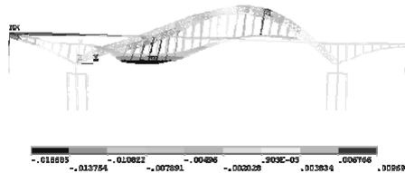
Figure 6: Deformed shape for half span loading
