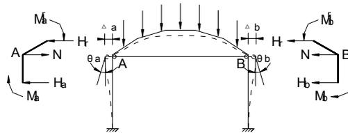
Figure 6: Simplified mechanical system under dead load
