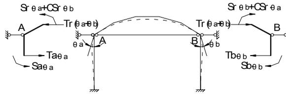
(b) Only rotation is allowed at joint A and B
