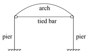
Figure 1: Rigid-frame tied through CFST arch bridge
