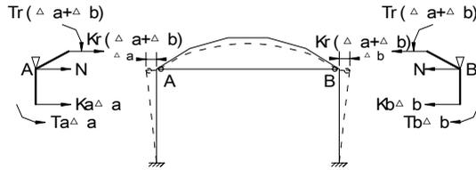
(c) Only displacement is allowed at joint A and B
