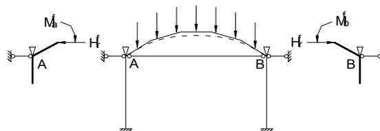
(a) No deformation is allowed at joint A and B
