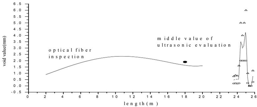
Figure 8: Arch crown void distribution of 8# tube
