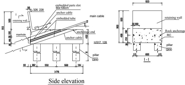
Figure 3: Layout of hoisting anchorage
