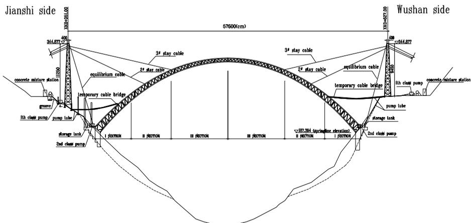
Figure 6: Layout of pouring concrete filled in tube
