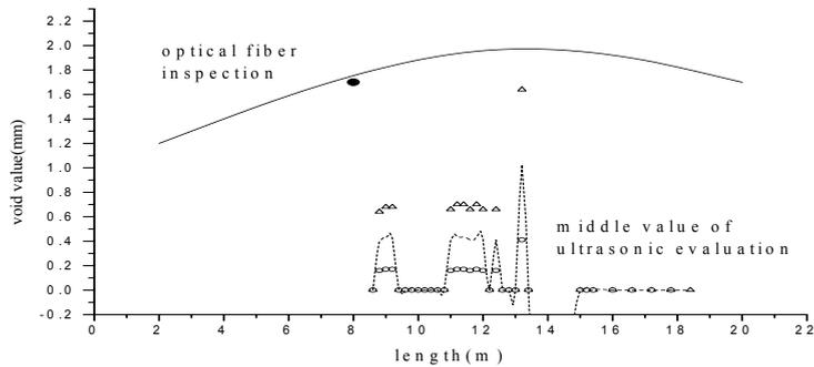
Figure 7: Arch crown void distribution of 6# tube
