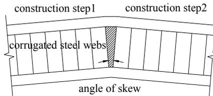
Figure 5: Angle of skew between two web segments
