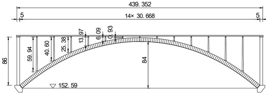
Figure 1 : Layout of the trial design (unit: m)
