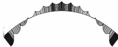
Figure 6 : Distribution of bending moment in corrugated steel webs arch under dead load
