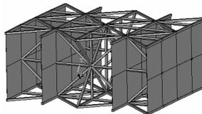
Figure 7 : 3-D FE model of a segment of the embedded scaffolding in the trial design bridge
