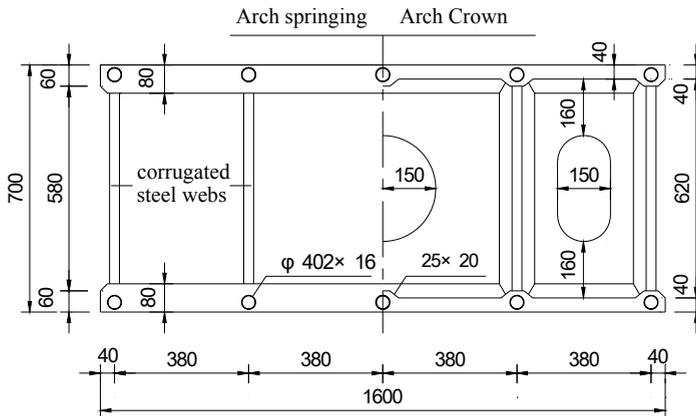
Figure 2: Arch cross section of the trial designed bridge (unit: cm)
