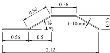
Figure 3:Dimensions of the corrugation profile
