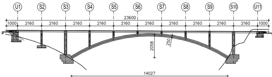
Figure 2: Longitudinal layout of Cetina River bridge
