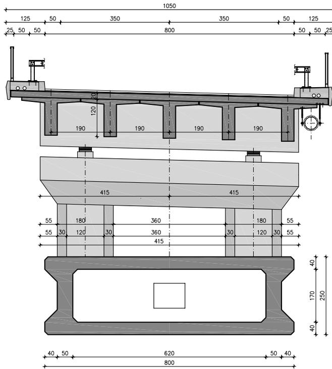
Figure 1: Arch and superstructure cross section of Cetina River bridge
