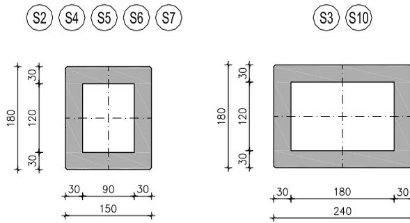
Figure 3: Column cross sections of Krka River bridge
