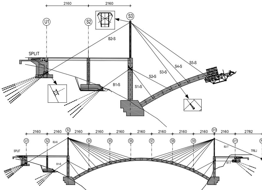
Figure 4: Arch construction by free cantilevering
