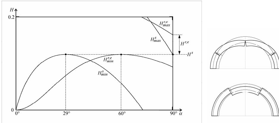
Figure 7 : Collapse condition for both mixed and sliding mechanism ( $K = 1.2205$ ,  $\mu = 0.309$ ).
