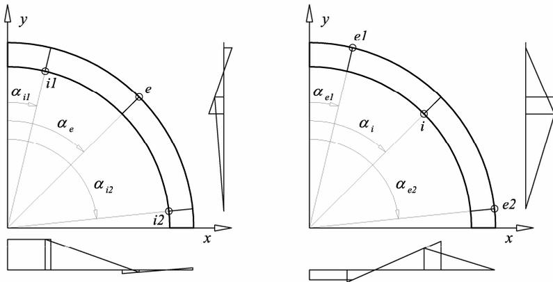
Figure 3 : The two rotational mechanisms with one degree of freedom.
