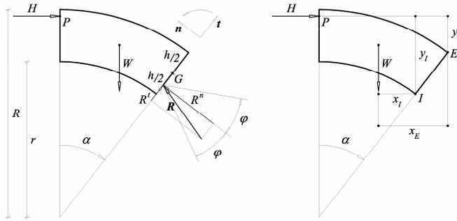
Figure 1 : Scheme of the generic voussoir of the arch.
