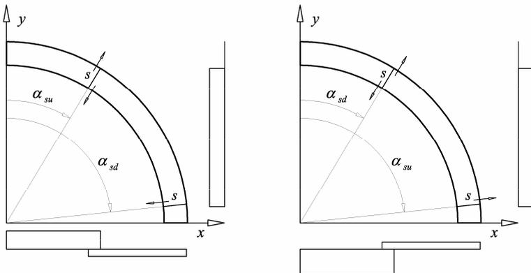
Figure 5 : The two sliding mechanisms with one degree of freedom.
