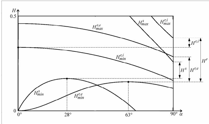
Figure 2 : Domains  $H^r$  and  $H^s$  for an arch with  $K = 1.35$  and  $\mu = 0.4$ .
