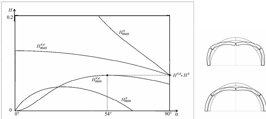
Figure 6 : Collapse condition for both rotational and mixed mechanism ( $K = 1.1136$ ,  $\mu = 0.395$ ).
