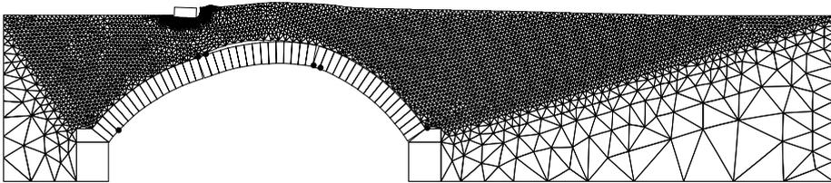
Figure 2 : Deformed shape of soil and arch (UB1)
