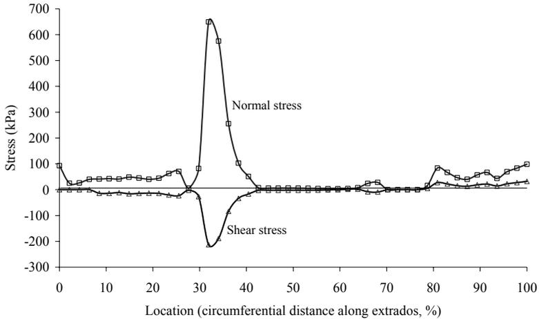
Figure 5: Shear and normal stresses on the extrados (LB1),  $\delta/\phi' = 0.33$
