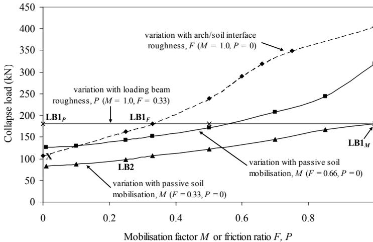
Figure 7: Variation in ultimate load capacity (lower bound) with different soil/arch interface properties, soil mobilisation factors and platen base friction properties. Soil mobilisation factors were applied only to passive side of arch (letters in brackets indicate the parameter plotted on the x-axis).
