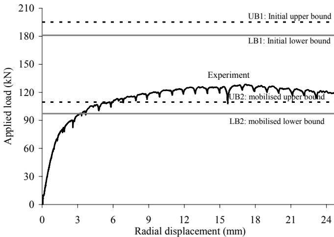
Figure 6: Predicted and experimental load vs. displacement responses for masonry bridge (LB1, UB1:  $M = 1$ ,  $F = 0.33$ ,  $P = 0$ ; LB2, UB2:  $M = 0.25$ ,  $F = 0.33$ ,  $P = 0$ )
