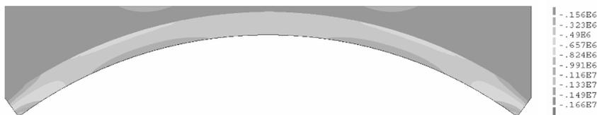
Figure 6 : Minimum compressive stresses depicted on the undeformed mesh for the dead weight of the bridge (values in [Pa]).
