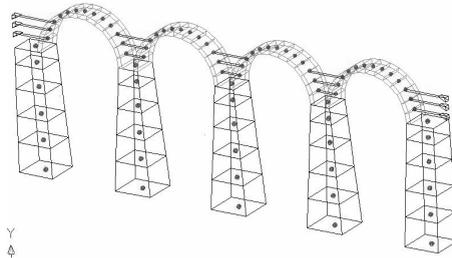
Figure 5: Masonry bridge mesh through mono-dimensional non-linear elements.
