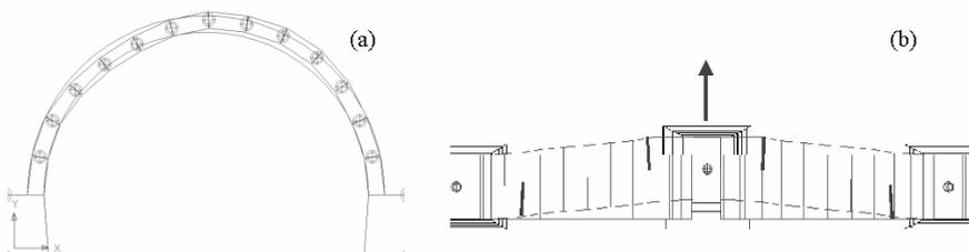
Figure 4: Damage mechanism schematisation: (a) in the arch thickness; (b) in the whole vault (top view).
