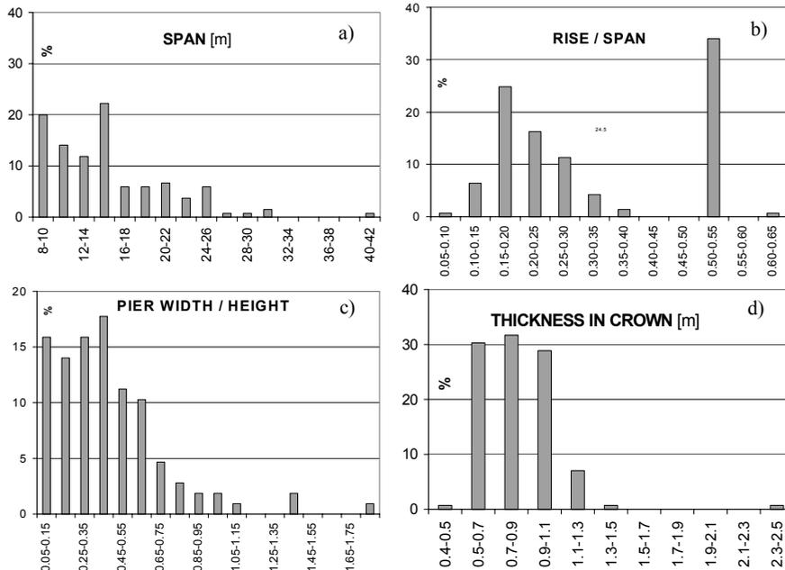
Figure 1: Statistical distributions: a) span length; b) rise/span ratio of the arch; c) pier width/height ratio; d) arch thickness in crown (Gambarotta *et al.* 2002).
