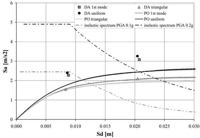
Figure 7: Cantalupo viaduct: comparison between static and dynamic procedures.
