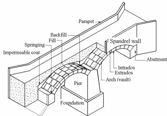
Figure 3: Axonometric section plane of a masonry bridge.
