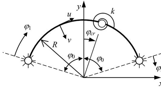
Figure 4 : Symmetric circular arch embedding a damaged section.
