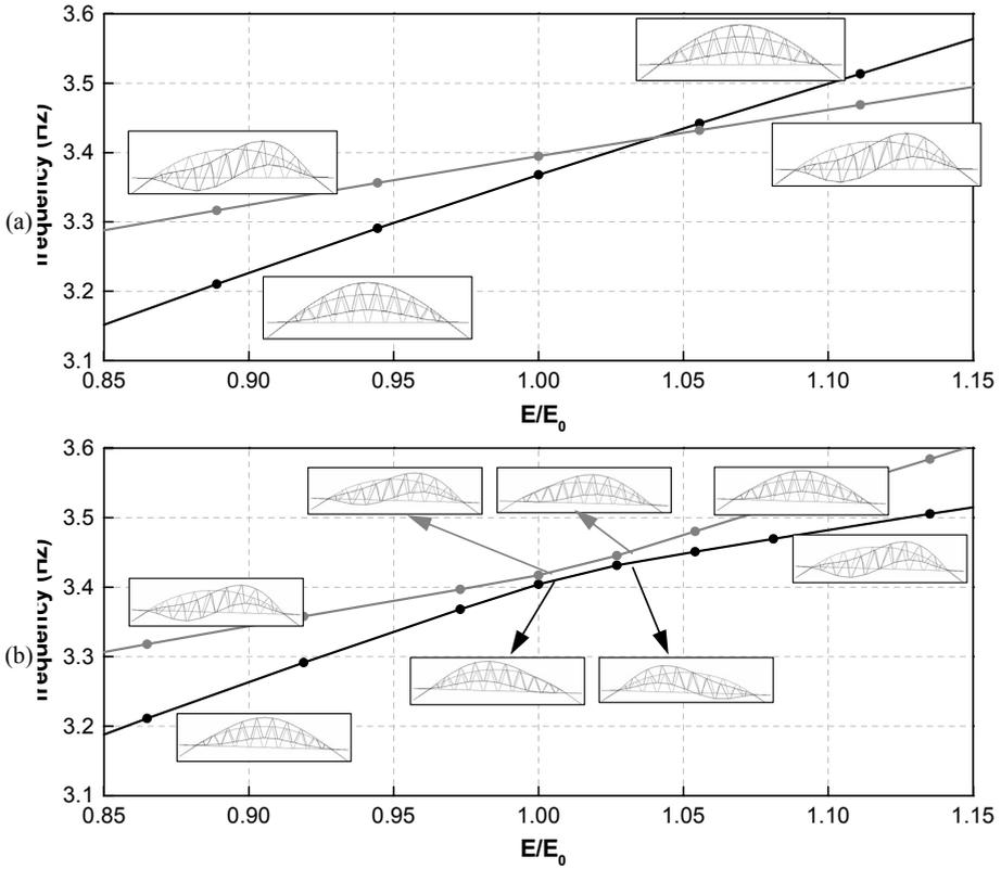
Figure 2 : (a) Crossing on a symmetric and (b) Veering on a non-symmetric arch bridge model.
