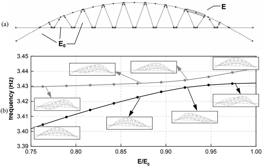
Figure 3 : (a) Damaged arch bridge model; (b) Veering on the damaged arch bridge model.
