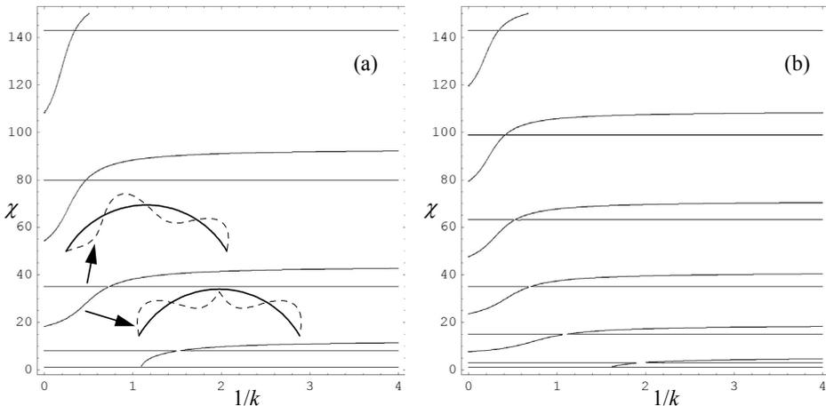
Figure 5 : Normalized eigenfrequencies vs flexibility of the damaged section for a symmetrically damaged arch. (a)  $\varphi_0 = \pi/3$ ; (b)  $\varphi_0 = \pi/2$ .
