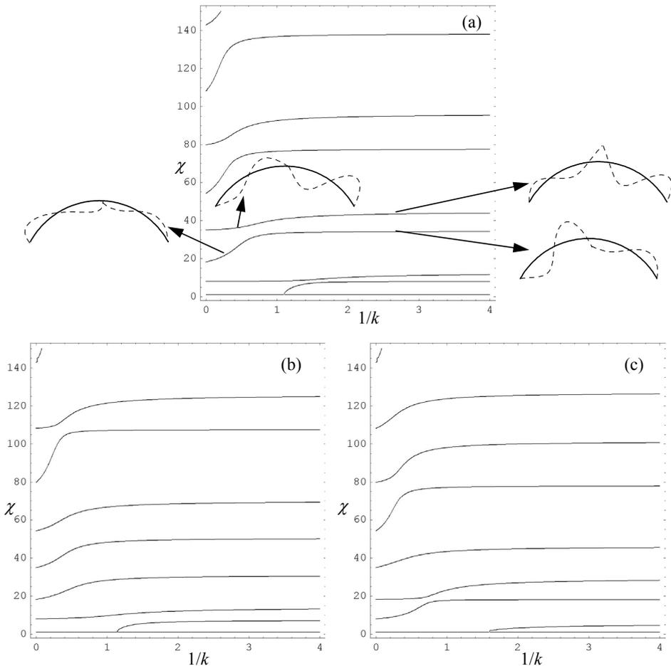
Figure 6 : Normalized eigenfrequencies vs flexibility of the damaged section for an unsymmetrically damaged arch with  $\varphi_0 = \pi/3$ . (a)  $\varphi_{cr} = \pi/72$ ; (b)  $\varphi_{cr} = \pi/24$ ; (c)  $\varphi_{cr} = \pi/8$ .
