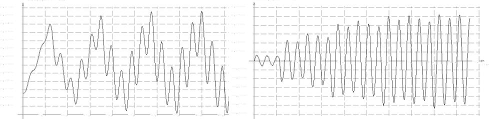
Figure 5 : Arch top displacements (left) and accelerations (right).
