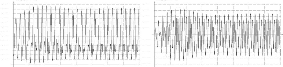
Figure 7 : Arch top displacements (left) and accelerations (right) for period of 2.8 s
