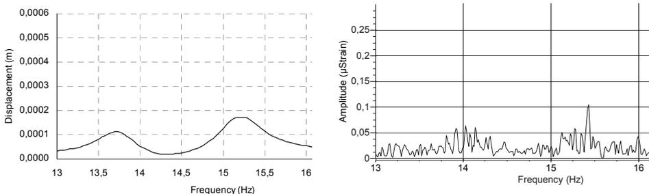
Figure 7 : Predicted and measured frequency response curve for near - optimum damper.
