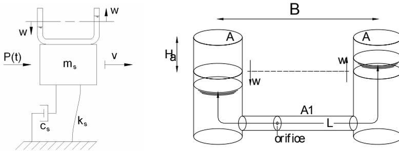
Figure 2 : STLCD fitted on a SDOF structure : notations
