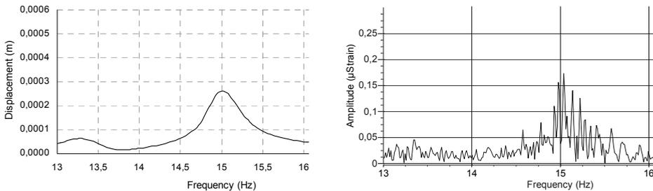
Figure 8 : Predicted and measured frequency response curve for non - optimum damper.
