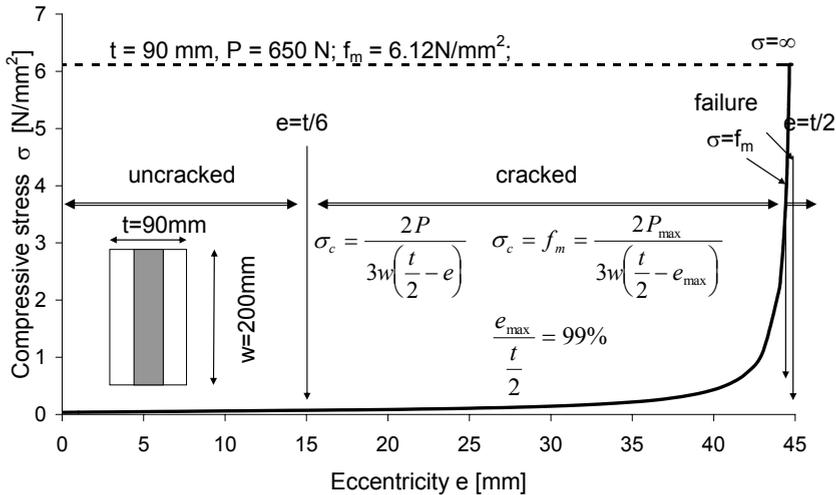
Figure 8: Compressive stresses in the mortar as a function of the eccentricity  $e$  of the thrustline in a cross-section for the material properties obtained for the pointed arch, using a Non-Tension Material behaviour
