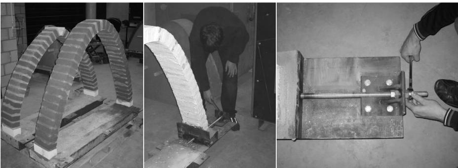
Figure 6: Pointed and parabolic arch, and setup for movable abutment
