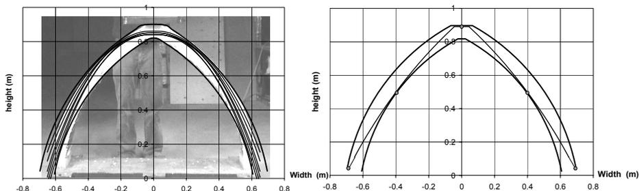
Figure 1: Location of thrustlines within the arch: (a) without external loading; (b) when the maximum vertical loading is applied and the load-bearing capacity is reached ( $F_v=550$  N)
