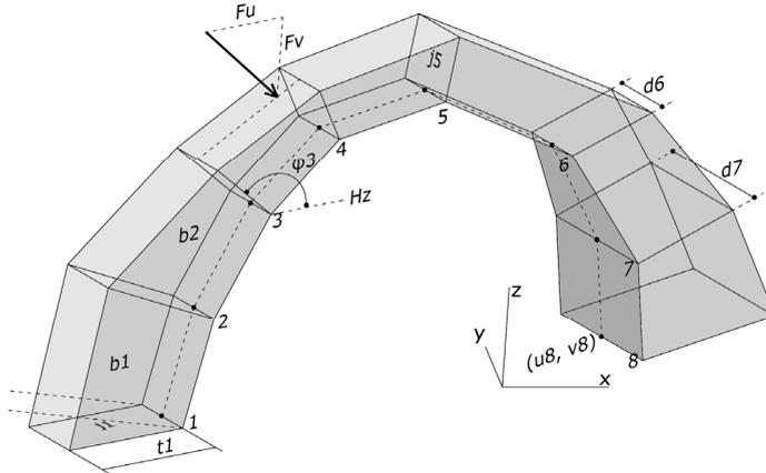
Figure 2: schematic view of an arch as defined in the *Calipous* computer program
