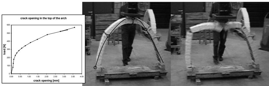
Figure 7: crack opening in the top of the arch – formation of 4 hinges at collapse of parabolic arch.
