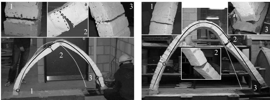
Figure 9: pointed and parabolic arch during displacement test, showing an asymmetric crack pattern.
